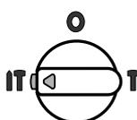
Position for **hammer drilling**
